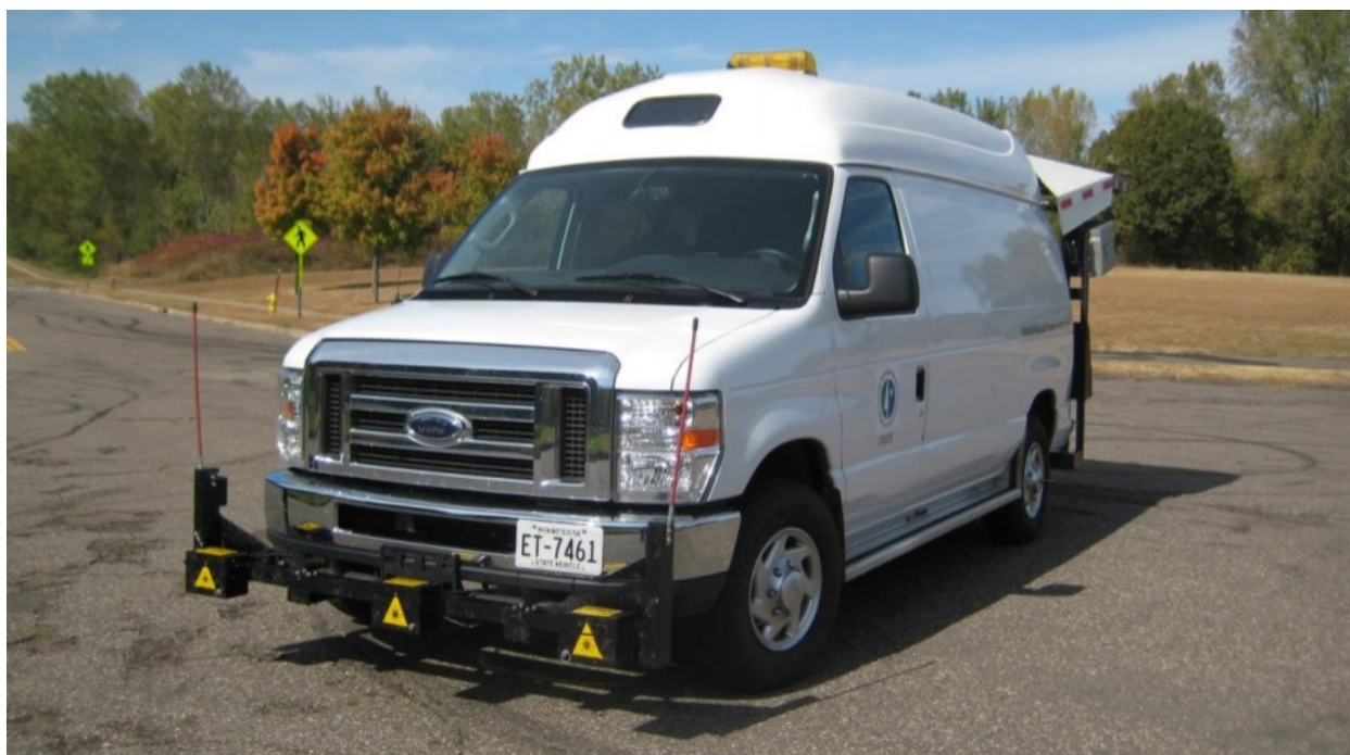
Figure 10.1 MnDOT digital inspection vehicle (DIV).
