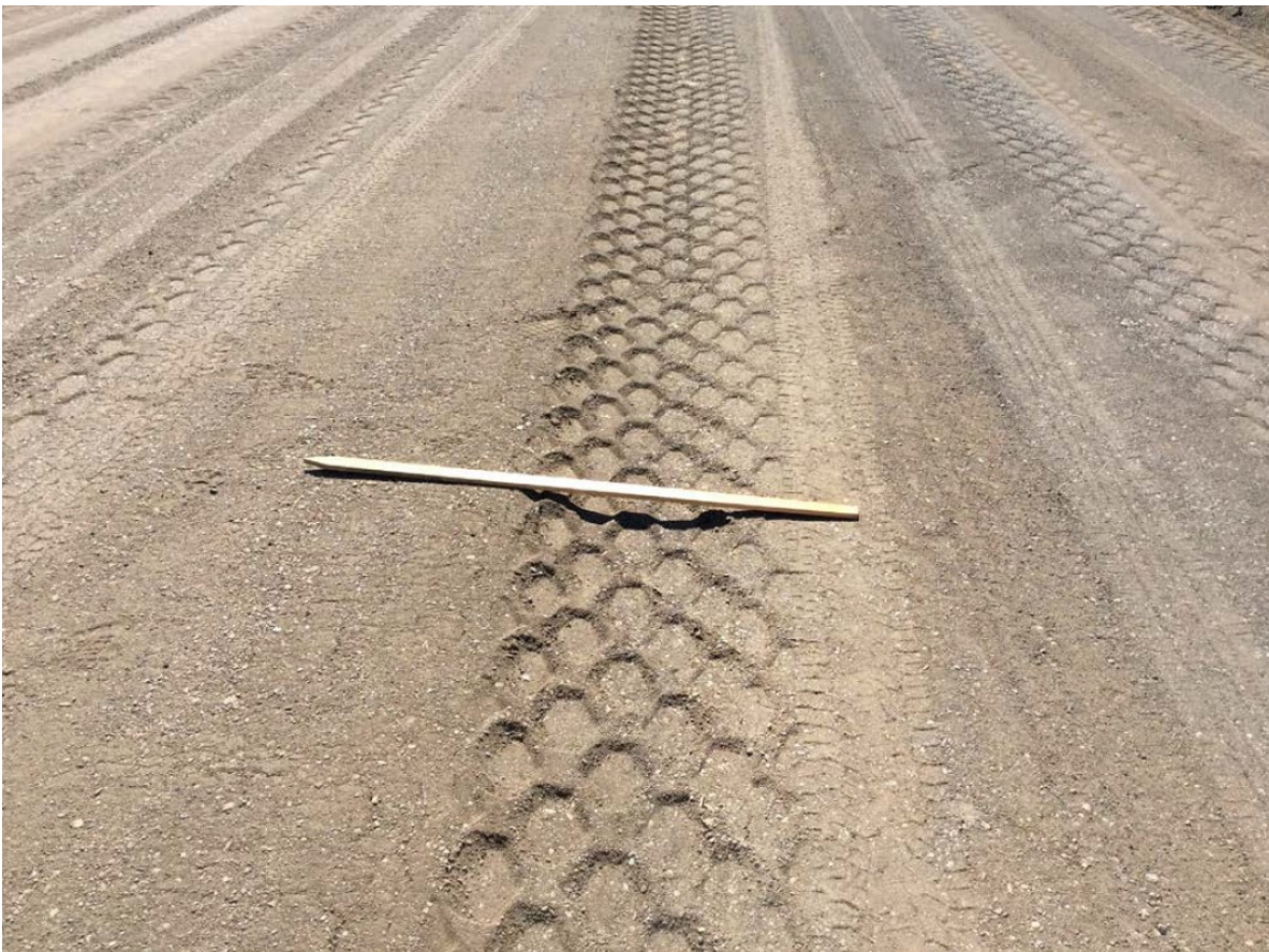
Figure 6.3 Rut in Cell 238 aggregate base due to passage of intelligent compaction steel drum roller.
